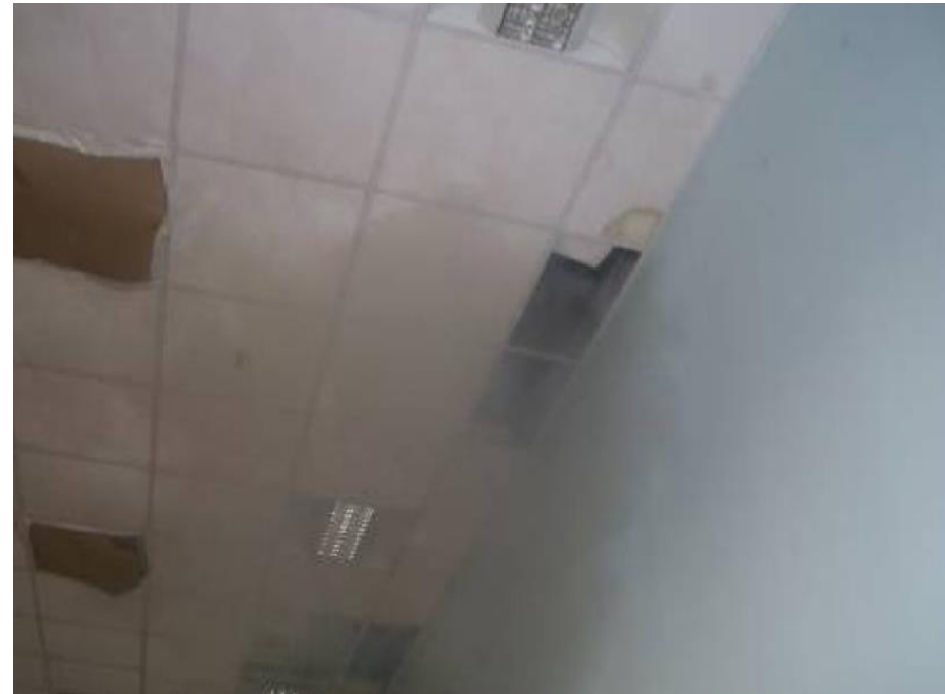
Test smoke pouring into dance studio from Wet area of building
