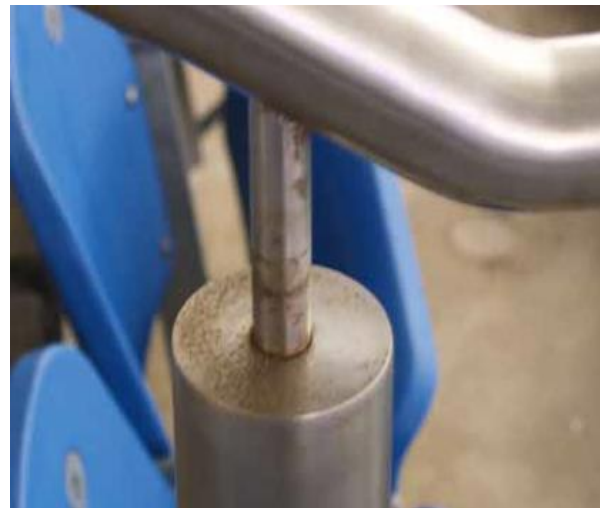
Examples of corrosion to steel fittings throughout the wet area found to be 304 grade steel as opposed to specified grade 316
