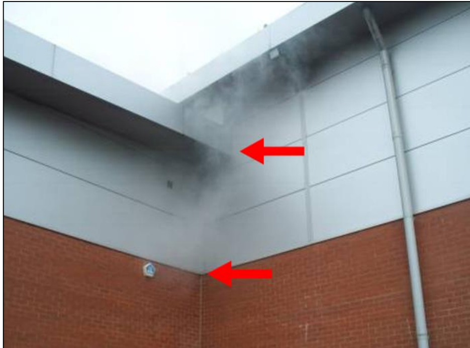
Test smoke rapidly escaping through eaves junction demonstrating lack of air-tightness
